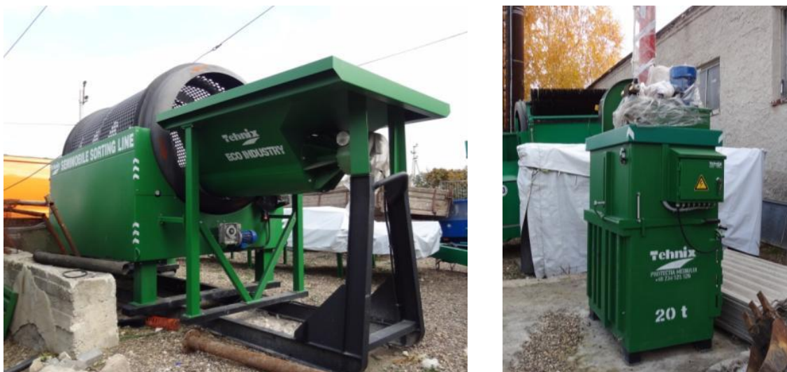
Figure 5-1: Sorting and bailing equipment (left: drum sieve, right: baler)
