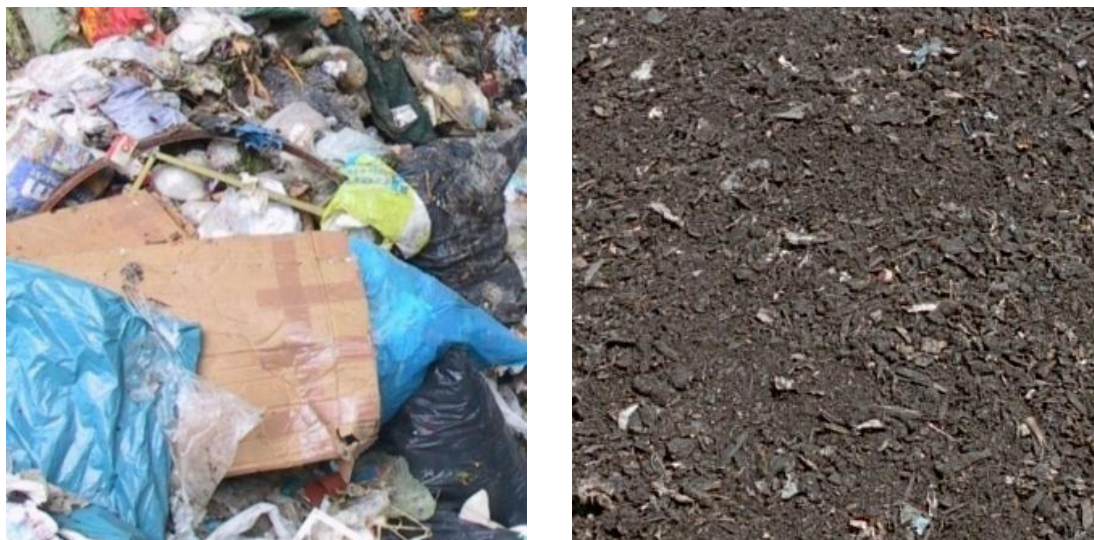
Figure 5-9: MSW prior (left side) and after (right side) biological treatment
