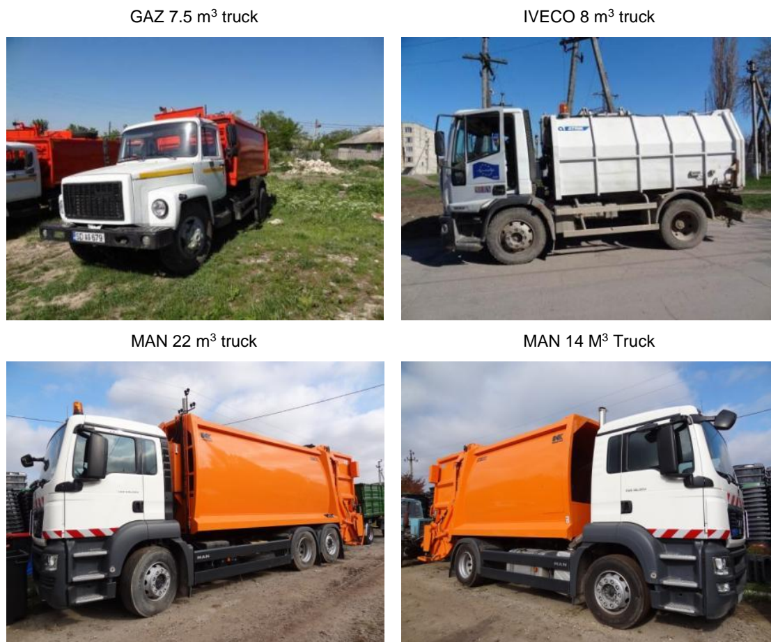
Figure 3-2: Type of compactor trucks used to collect the waste in the project area
