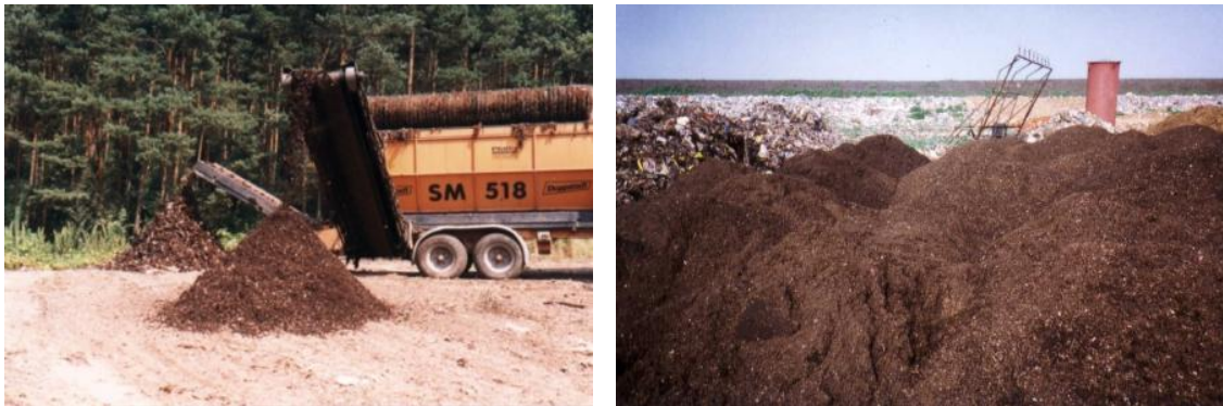
Figure 5-10: Screening of SB (left) & segregation of methane oxidation layer material (right)
