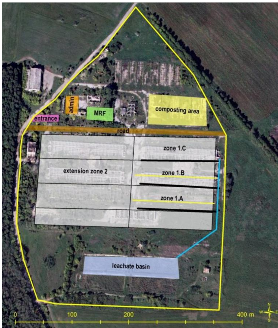
Figure 5-7: Conceptual design of enhanced transitional landfill – site map
